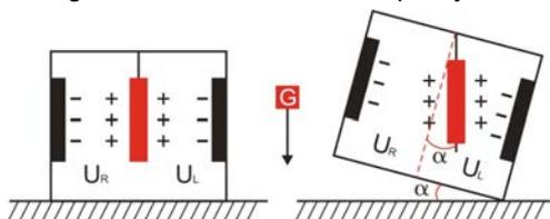
$U_R, U_L$  Respectively is the pendulum left plate and the right plate corresponding to their respective voltage between the electrodes, when the tilt sensor is tilted,  $U_R, U_L$  Will change according to certain rules, so  $f(U_R, U_L, )$  On the inclination of  $\alpha$  function:
