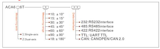
E.g: ACA616T-10-232: Single-axis/Standard /±10°Measuring range/RS232 output
